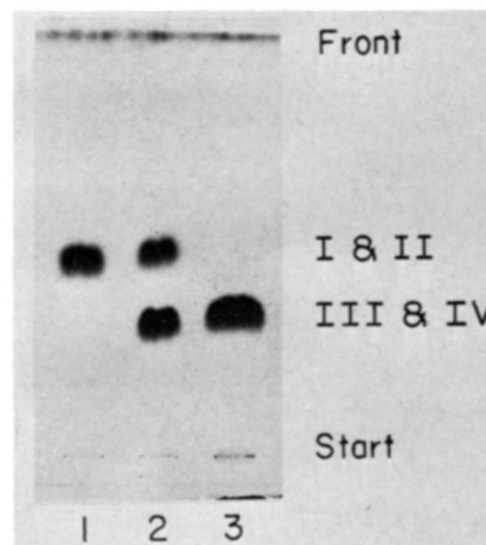
FIG. 3. Argentation TLC of triacetyl LCB. 1, monoenic triacetyl LCB from plasma sphingomyelins; 2, triacetyl LCB derived from partial hydrazine reduction of sphingadienine triacetate. 3, triacetyl sphingadienine derived from plasma sphingomyelins. The plate was developed with chloroform-methanol 98:2.
